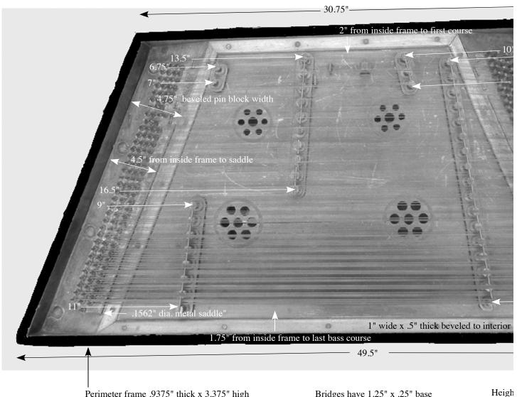
Perimeter frame .9375" thick x 3.375" high Back is 1.25" thick and extends 1/2" beyond the perimeter of the frame (measurements shown here)
